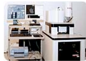
This is one of many SEMs specifically designed for the rapid characterization of particles. Source: McCrone Associates Inc.
