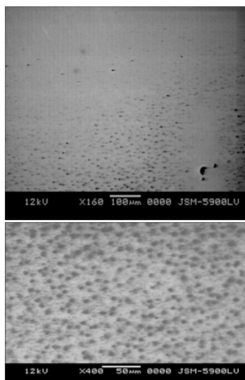
Figure 2 and Figure 3: Fine pitting on the glass surface of vials demonstrates tapering and enlargement of pits.
