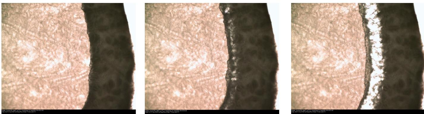
The sample pictures above, courtesy of Dr Zixin Huang, show the freeze drying process of 5% sucrose solution. The collapse of the product can be visualised and the temperature recorded, a parameter critical for the freeze drying process.
