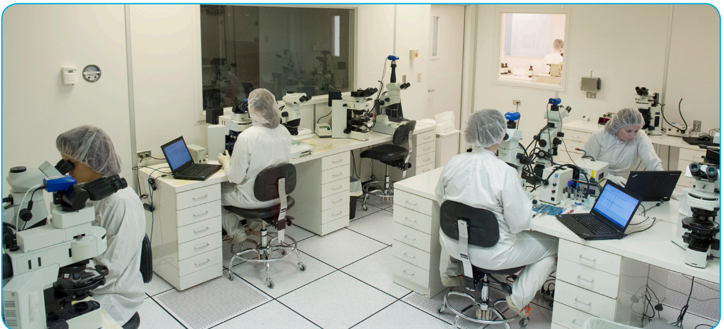
Microscopists isolate particles and prepare samples in an ISO Class 5 cleanroom at McCrone Associates.
