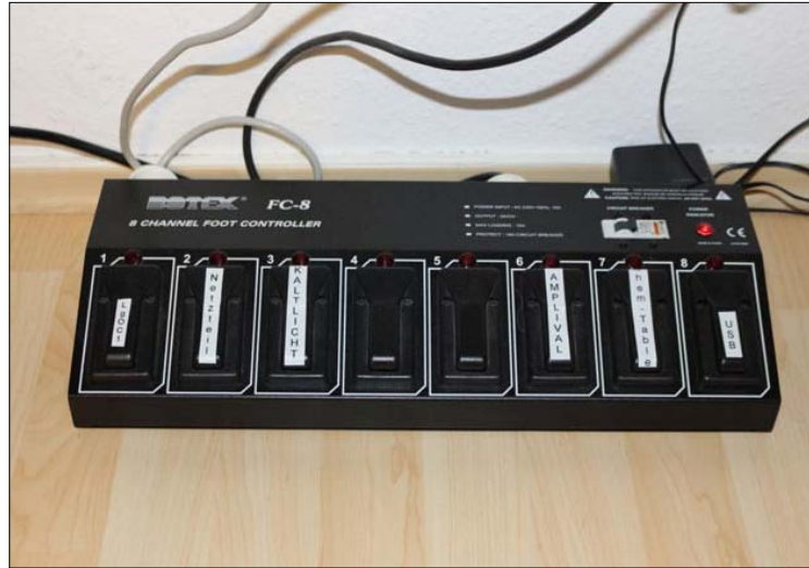
FIGURE 6 Foot controller, for illumination sources switching.
