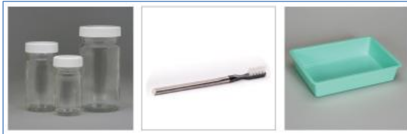
Figure 2: Supplies needed to collect diatoms are airtight glass jars, a toothbrush, and a plastic tray.
