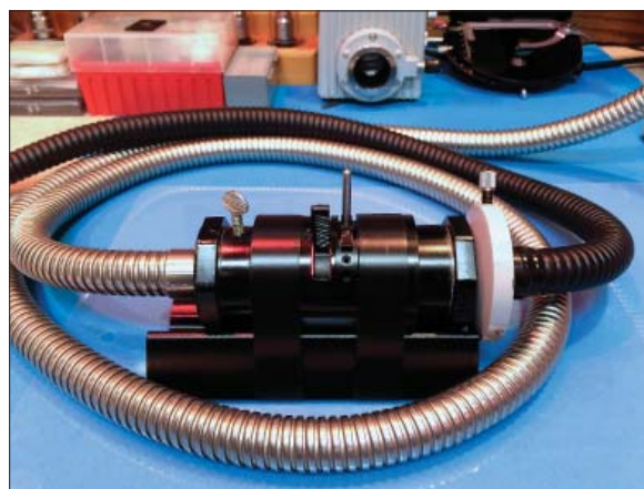
FIGURE 7 In-line filter holder, holds two filters.
