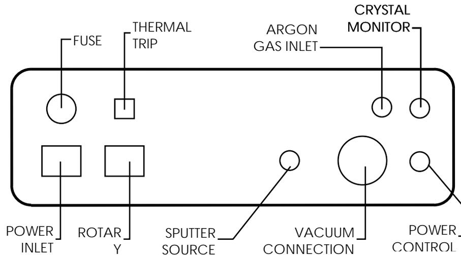
The high voltage power cable from the rear panel (*SPUTTER SOURCE*) to the sputtering head is permanently wired for safety. The output is also controlled by a protection circuit linked to the Pirani vacuum gauge: The high voltage output cannot be energized until the vacuum is better than 0.4mb. (If the Pirani gauge becomes faulty the supply will not energize and the fault condition will be indicated by the *mb* light flashing and the vacuum meter needle being off-scale in either direction).
