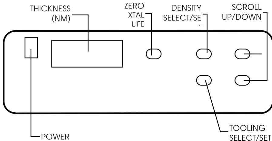
The thickness monitor calculates the thickness of deposit every tenth of a second and displays the result in nanometers on the digital *THICKNESS* display. It detects the frequency shift and uses the *DENSITY* and *TOOLING* values stored into memory. Four sets of values can be stored under *DENSITY* and *TOOLING*.
