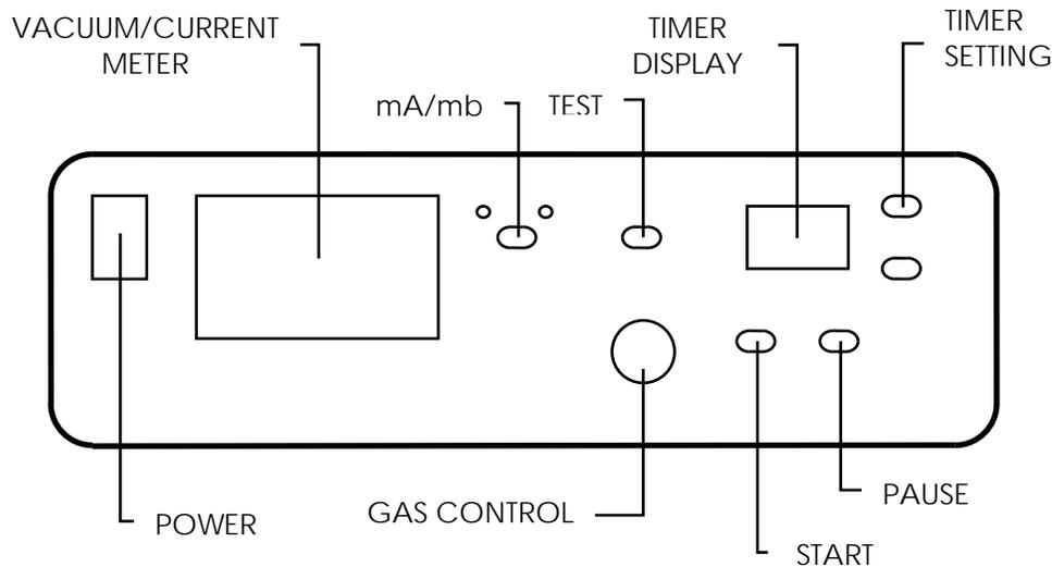
Rotating the gas control knob in a counterclockwise direction allows gas to enter the sputter chamber through a gas metering valve. Sputtering is usually carried out between 0.05mb and 0.10mb (see Sections 5.1/5.2). Power output can be checked before starting the coating cycle by pressing *TEST*. Power adjustment is on the rear panel (see next page).
