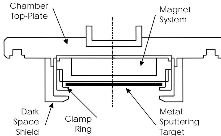
(57mm dia x 0.1mm thick) is held by a threaded clamp ring. The dark space shield must be removed before the target can be changed.
