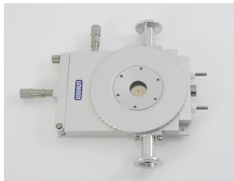
*The THMS350V heating and freezing vacuum stage*
