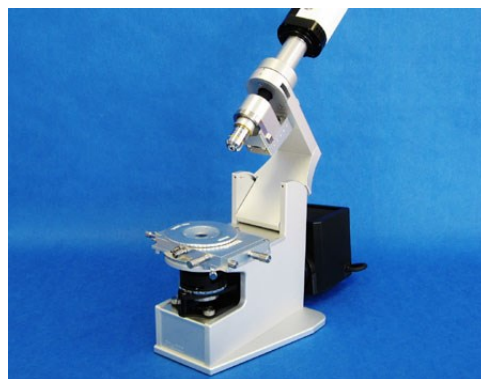
Linkam Imaging Station. Optics are tilted back to allow easy access to sample
