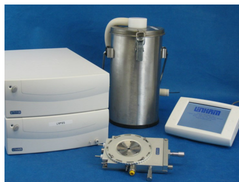
THMS600-PS Pressure System with T95-LinkPad and LNP95 controller
