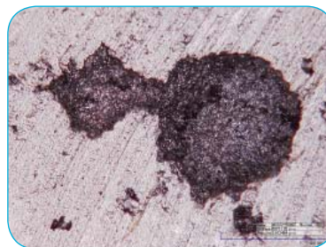
Image of a hole in cast iron. 50X.
