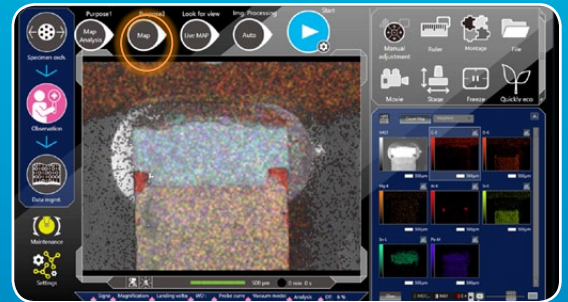
Embedded EDS option with live analysis.
