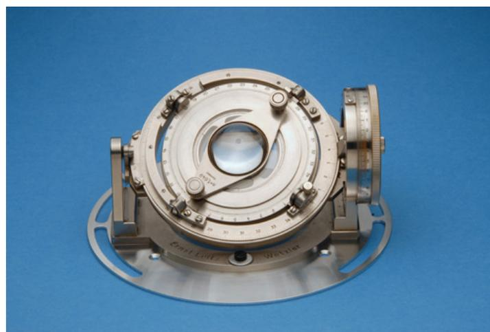
Figure 9 (below) shows the Leitz 4-axis universal stage mounted on its adapter plate, now affixed to the Olympus stage using two knurled thumbscrews M3.0 x 0.50; fiber washers were chosen for smoother sliding during the centering operation. This completes the U-stage-to-Olympus-stage modification (the microscope stage has been removed from the microscope for clarity).
