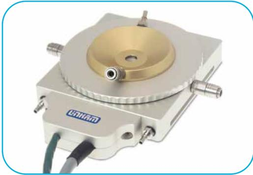
Gain complete understanding of sample behavior at extreme high temperatures with our TS1500. This system can be integrated with light microscopy, X-ray or Raman to give you all the data you need to characterize fluid inclusions, determine high melting points or investigate complex materials. The TS1500 can uniformly heat samples at 200°C per minute, all the way up to 1500°C.
