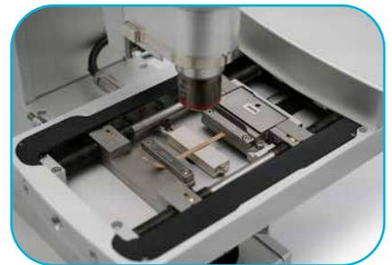
This system is a new, improved version of the TST tensile stage with increased sensitivity and resolution. The modular design allows you to have an additional level of control over your experiments with the ability to change grips, heater types and force beams. It offers a flexible upgrade and customization path. Additional options accommodate a wide range of different samples and applications.
