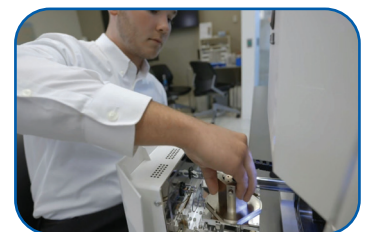
Loading a sample in the JEOL JCM-7000.
