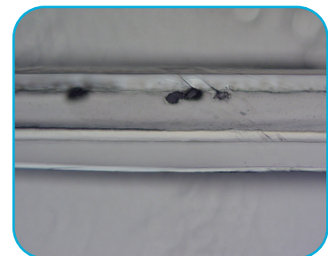
Debris inclusion embedded in a multi-layer film.
