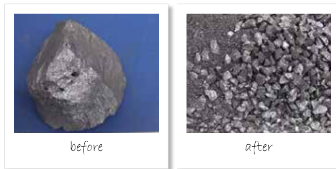
Fig. 2: Silicon sample before and after crushing in a jaw crusher
