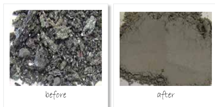
Fig. 4: SiC sample before and after pulverization in a mixer mill
