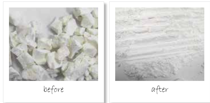
Fig. 4: Composite ceramics before and after pulverization in a planetary ball mill
