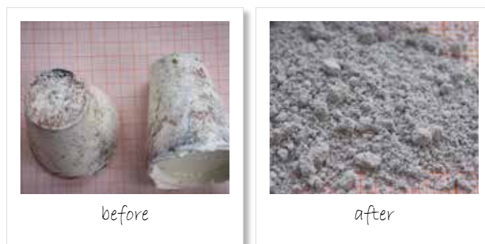
Fig. 2: Ceramic cones before and after size reduction in a jaw crusher
