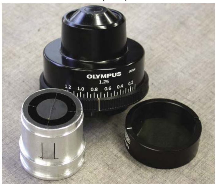
Figure 7-Photograph of the Olympus Abbe condenser and the insert for critical darkfield dispersion staining with the 40X 0.65 NA Olympus objective.
