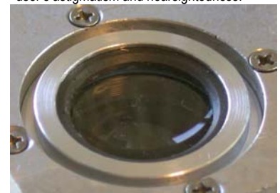
Figure 5: Close-up view showing the recess for the Coolpix camera lens flange to minimize the gap between the eyepiece and front of the camera lens.
