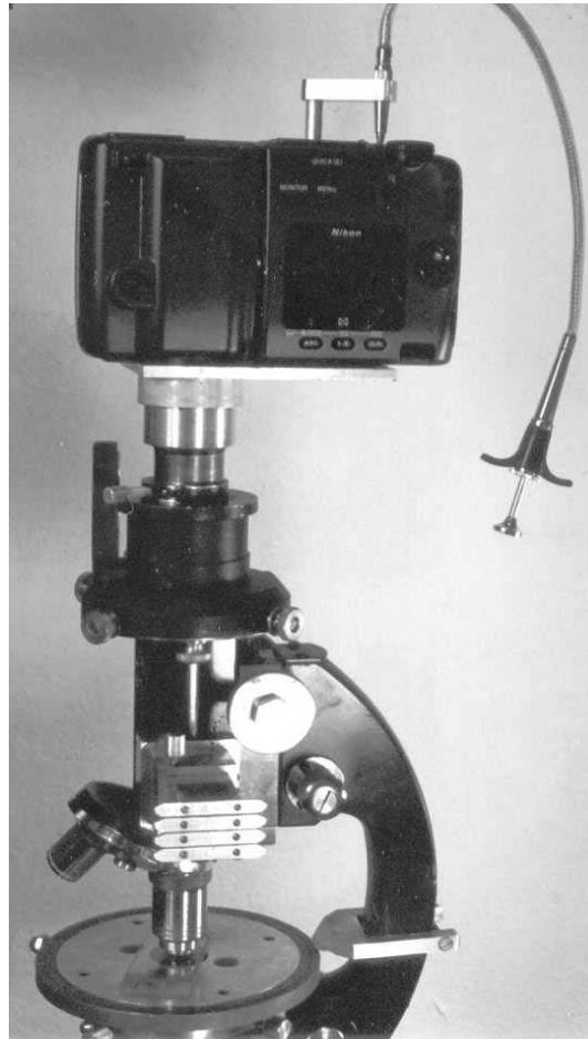
Figure 3: Polarized light capable Monolux microscope with a Nikon Coolpix camera mounted on the eyepiece.
