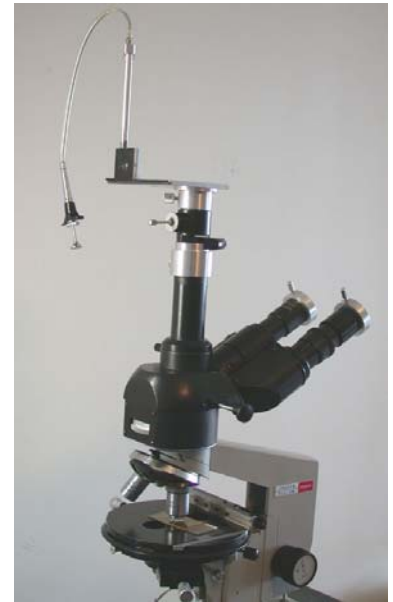
Figure 4: Mounting bracket for a Nikon Coolpix camera attached to a LOMO Edupointer eyepiece in the trinocular phototube on a LOMO Biolam microscope with eyecaps on the binocular eyepieces to correct for the user's astigmatism and nearsightedness.
