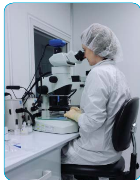
Samples are prepared in McCrone Associates' cleanrooms, which are certified to ISO 14644 Class 5 standards.
