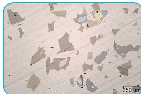
Glass delamination on filter, the same field of view as the image above, 60X magnification, but using coaxial illumination.
