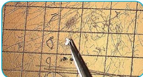
Using a tungsten needle, the washed sample is transferred to a beryllium stub.
