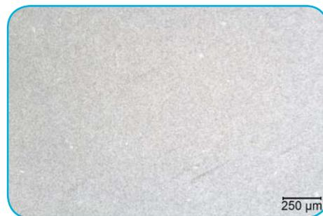
Glass delamination on filter, stereomicroscope, 60X magnification, oblique illumination.
