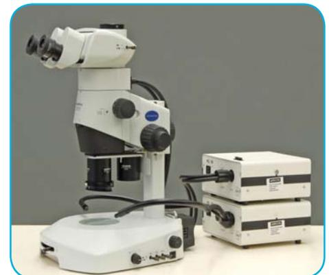
A stereomicroscope configured for use with transmitted, coaxial, and oblique light.
