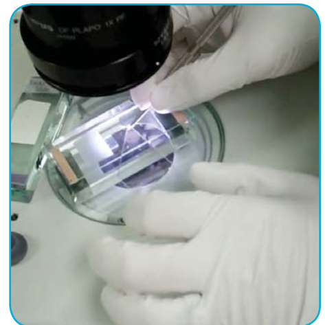
Kristen demonstrates how to use a wedge slide to press a polymer sample.
